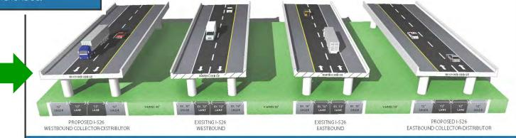
INTERSTATE 1-526 | EXISTING 1-526 2-LANE VIADUCTS RETAINED AND PROPOSED 2-LANE STRUCTURES TO OUTSIDE
