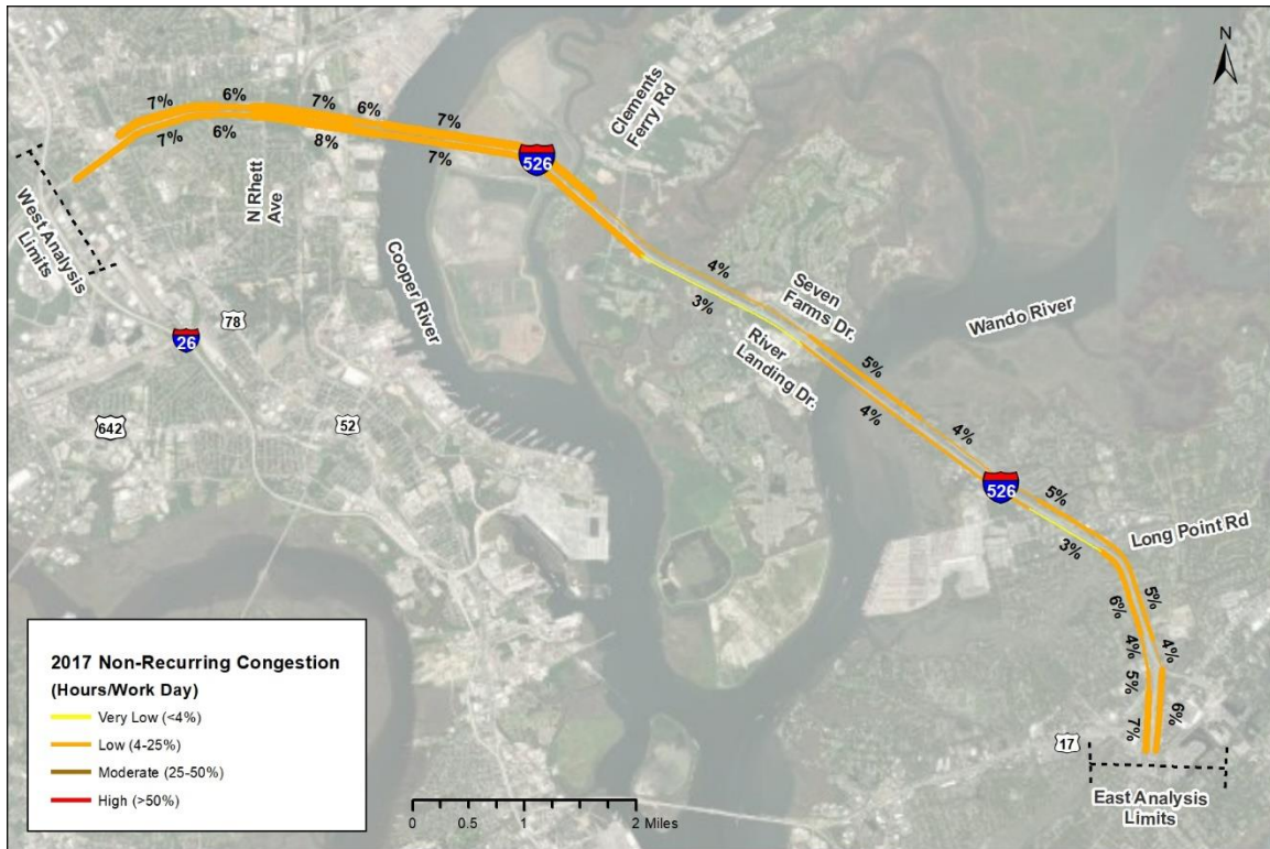
Figure 3-3: Frequency of Moderate or Worse Non-Recurring Congestion (% of Time Periods with TTI > 1.1 & SND < -1.5 ) 2017
