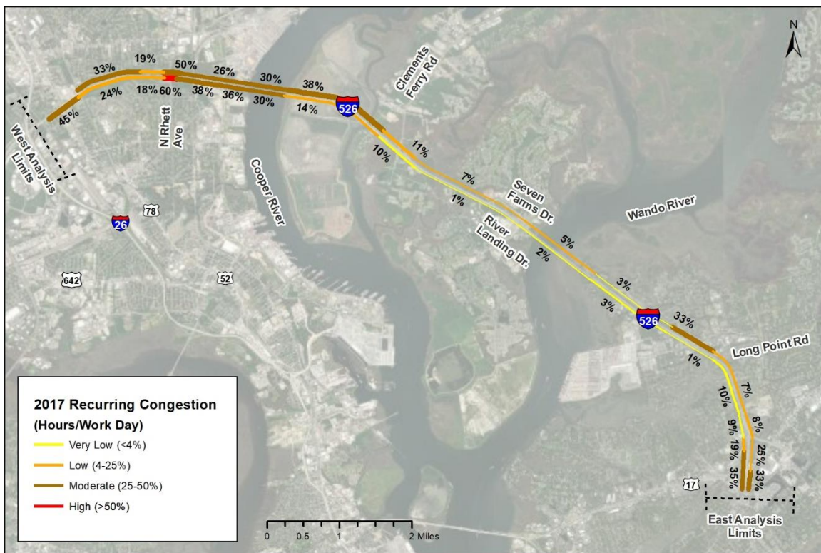
Figure 3-2: Frequency of Moderate or Worse Recurring Congestion (% of Time Periods with TTI > 1.1 & SND > -1.5 ) 2017
